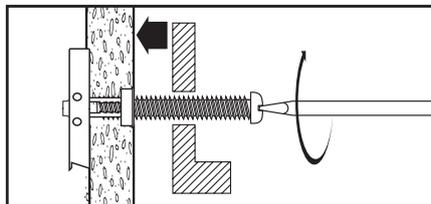
6.) Position the fixture. Insert the bolt through the fixture and tighten. The minimum bolt length should be at least 1/2" longer than the combined wall and fixture.
