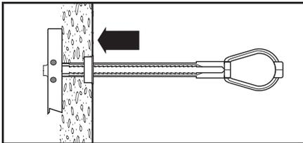
3.) Slide the plastic cap forward until the flange is seated flush against the work surface.
