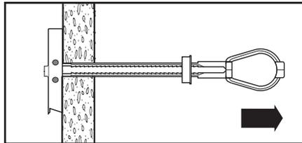
4.) Pull the wing firmly against the inside wall of the hollow material.
